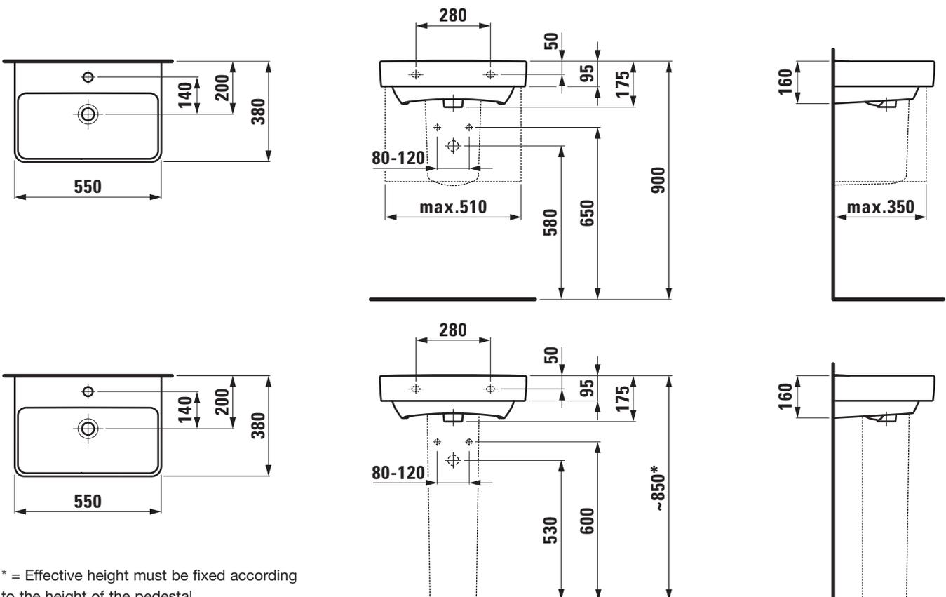
\* = Effective height must be fixed according to the height of the pedestal.
