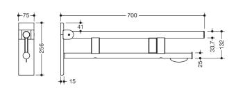
Abmessungen in mm
