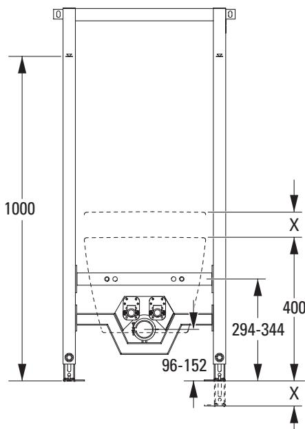
The bidet frame must be adjusted to a ceramic height of 400 mm. If the upper edge of the ceramic should be suspended higher, the feet of the frame must be adjusted accordingly prior to the installation.
